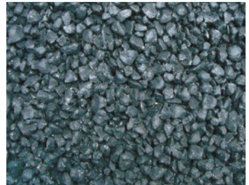
Drainage type Porous Pave
